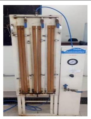
U tube manometer three different fluids
