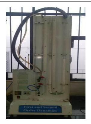
Second order system (water-mercury manometer)
