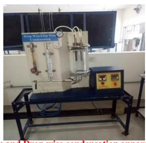
Film and Drop wise condensation apparatus
