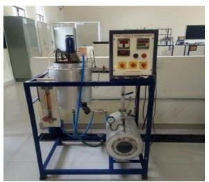
**Heat Transfer in Agitated vessel**
