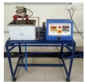
Unsteady state heat transfer by lumped capacitance
