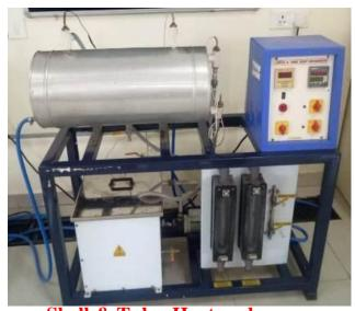
**Shell & Tube Heat exchanger**
