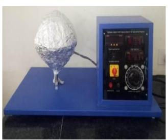
Thermal conductivity of an insulating powder material
