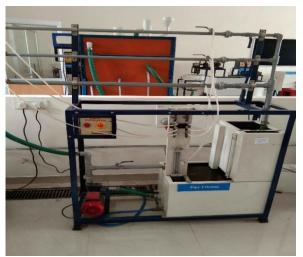
**Pipe Friction Apparatus**
