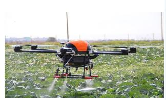
An agricultural drone is an unmanned aerial vehicle applied to farming in order to help increase crop production and monitor crop growth. Sensors and digital imaging capabilities can give farmers a richer picture of their fields. This information may prove useful in improving crop yeilds and farm efficiency.
