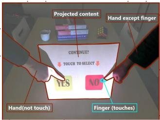
The system only requires a single camera attached just below the projector, and the system's developers say it works well no matter what you want to project.
