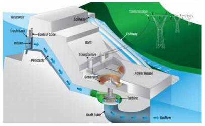
Figure 4. Hydroelectric power plant system
