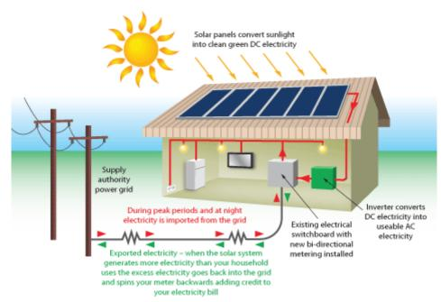
Figure-5: Grid-connected rooftop solar system Source: https://springviewz.com/solar-power-systems/
