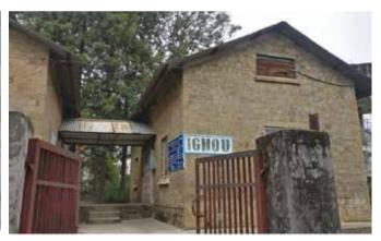
Figure-12: IGNOU building with small roof area and inappropriate orientation Source: Rooftop Solar detailed project report
